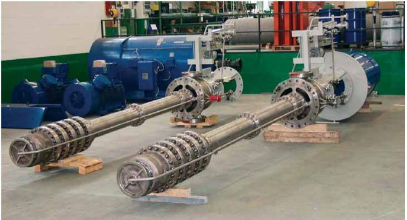
VBN pumps in Gabbioneta test room
